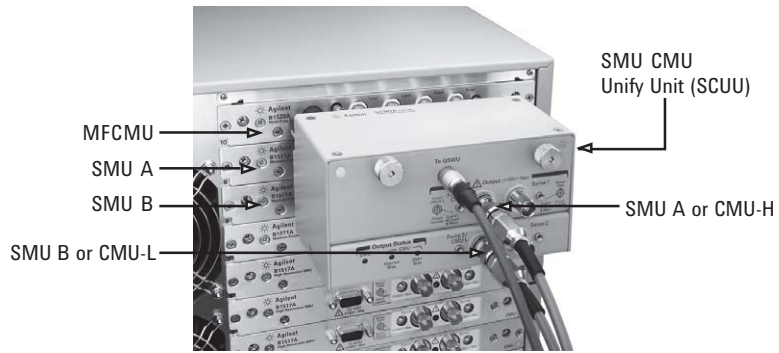
Figure 4. Accurate IV and CV measurement setup using SMU, MFCMU and SCUU.
