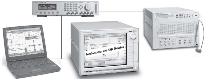
Figure 9. B1500A using an external PC to control analyzer measurement resources and external GPIB instruments. The built-in PC controller, touch-screen and GUI are disabled.
